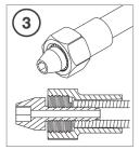
Pull the hose connector (A) towards the barb (B) making sure the thread is fully forward of the hose. (See cross section bottom left)
