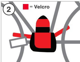
It can be adapted to fit your frame and motor shape by using the velcro straps. Correctly mounted the **Fibrax Motor Cover** fits tightly around the motor and frame and doesn't cause any scratches, which could occur when using a loose fitting cover.
