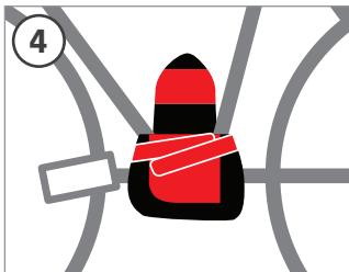
The **Fibrax Motor Cover** is not made to keep the motor dry but prevents the direct impact of spray water. The holes in the bottom of the cover allow the drainage of any entering moisture.
