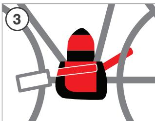
The **Fibrax Motor Cover** is for protection during transport and has to be taken off before using the e-bike.
